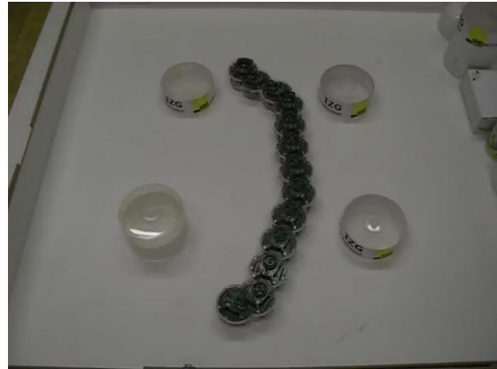
Fig. 1. Stroboscopic image of the arena with a moving e-puck robot and obstacles.
