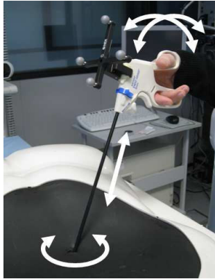
Fig. 1. The four free degree of freedom of a laparoscopic tool.
