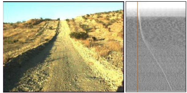
Fig. 7. Example of a non-flat ground V-Disparity image.
