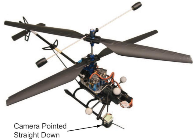
Fig. 5. The Blade CX2 helicopter that was used for the experiments. It is a coaxial helicopter with a rotor diameter of 34.5 cms, a height of 18.3 cms and weighs approximately 220g (with battery).
