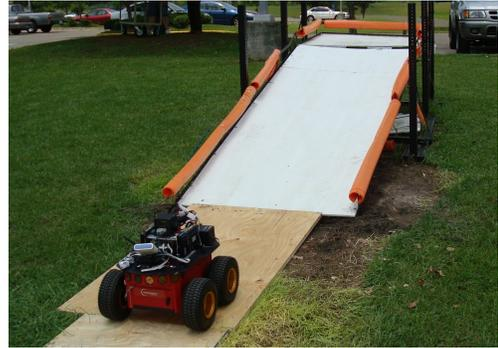
Fig. 4. Modified Pioneer 3-AT entering a white-board ramp
