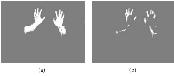
Fig. 5. Result of finger extraction using binary morphology. (a) Binary image of two hands, (b) Result subtracting (a) from the morphology image of (a).
