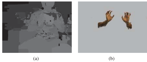
Fig. 4. (a) Disparity image generated using the graph-cut method, (b) The hand extraction result.
