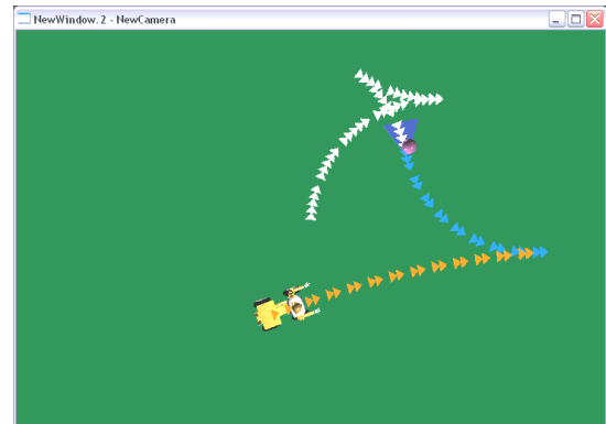
Figure 7. PIGI display for Centaur showing paths paths from the Predictor (shaded) and the Explorer (white). The small ball at the end of the path from PRED marks the location of the final expected state for all committed drive tasks. EXP paths start from there.
