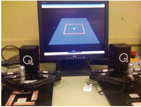
Fig. 3. Picture of the collaborative haptic training experimental setup.
