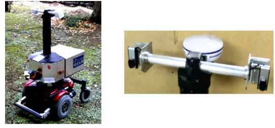
Fig. 6. Outdoor mobile root : Infant-Pro & Stereo camera rig
