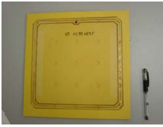
Fig. 13: IC Tag on guidance block
