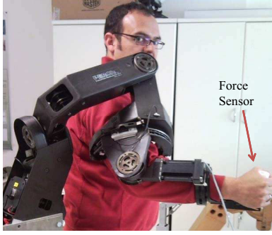
Fig. 2. L-Exos platform is worn by user
