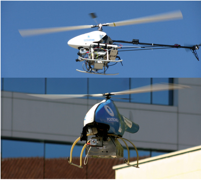
Fig. 1. Up: COLIBRI III Electric helicopter with a stereo camera system. Down: COLIBRI I Gas power helicopter
