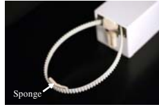
Fig. 2. Prototype I detail view: the active grasping part
