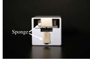
Fig. 3. Prototype I detail view: the passive grasping part
