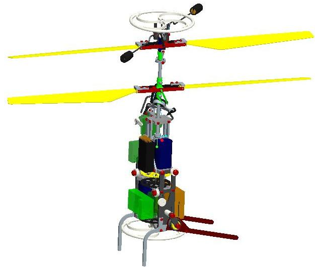
(b) The robot in its flight mode
