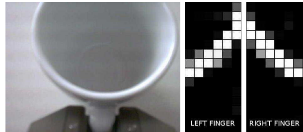
Fig. 1: Left: A manipulation robot with touch-sensitive finger tips learns to distinguish a large set of objects (here: a coffee mug) solely by using its touch sense. In the image, both the cup and (at the bottom end) the two fingers of the robot's gripper are visible. Right: Tactile images of the sensor array in the left and the right finger. The robot is perceiving the handle of the cup.
