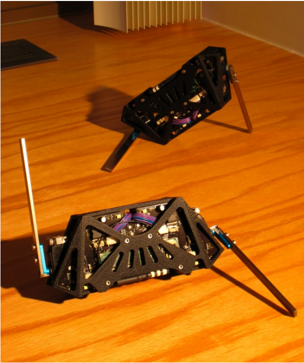
Fig. 1. Two Adelopod tumbling robots shown next to each other.
