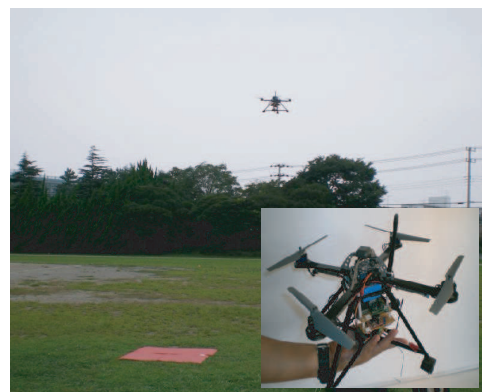
Fig. 1. The quadrotor MAV during vision-based autonomous flight. In the right corner, is the quadrotor MAV prototype used in the experiments. The small size and robustness of the vehicle can be potentially utilised in various area of applications
