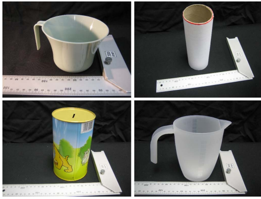
Fig. 6. Cylinder-like objects. Properties (radius x height, weight) from left to right and top to bottom: Cylinder1(110x80, light) Cylinder2(65x215, light) Cylinder3(105x75, heavy) Cylinder4(115x50, light)
