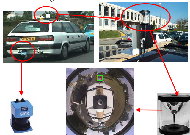
Fig. 1. The ADAS perception solution on the vehicle and an example of omnidirectional image.
