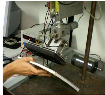
Fig. 5. Prosthesis foot orientation estimator providing estimates to a controller responsible for keeping foot parallel with respect to ground.
