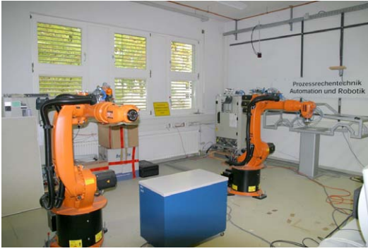
Fig. 4. Laboratory at the IPR: 2 KR16 robots, a 4 \times 4 \times 2m^3 volume is covered by the infrared tracking systems. Devices shown in Fig. 2 and Fig. 3 can be used in this volume to control the robots.
