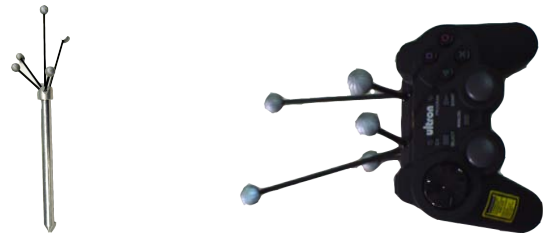
Fig. 3. Input devices - They are tracked via a tracking system by the sphere markers. Left: General input device with different kind of knobs, sliders and buttons installed; right: pen-like input device.
