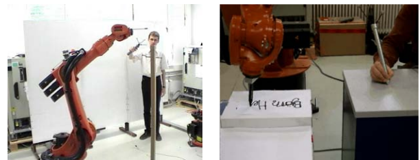
Fig. 11. Video scenes - Left: Jogging the robot with the input device shown in Fig. 2; right: Writing with a virtual pen - The manual movement is executed and copied at the same time by the robot.
