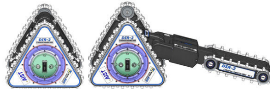
Fig. 3 Folding state (left) and Extended state (right). Link B and the straight crawler can be completely folded inside the triangular crawler unit in the side view.
