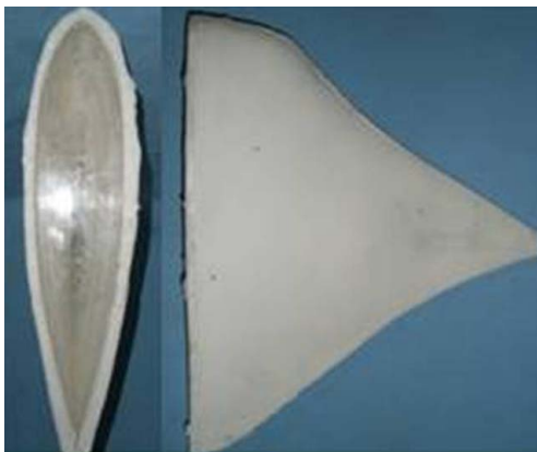
Fig. 4. The right part of the whole-flexible body before dressing, showing with the midsection and the cavity
