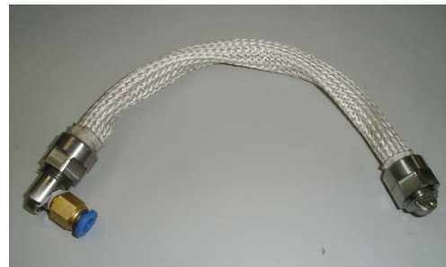
Fig. 5. The self-made pneumatic artificial muscle
