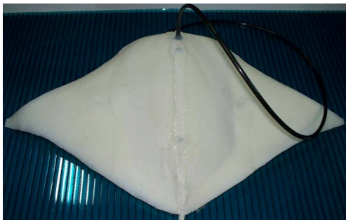
Fig. 8. The flexible robotic fish with the soft air tube
