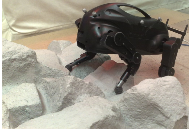
Fig. 1. The LittleDog quadruped robot on rocky terrain
