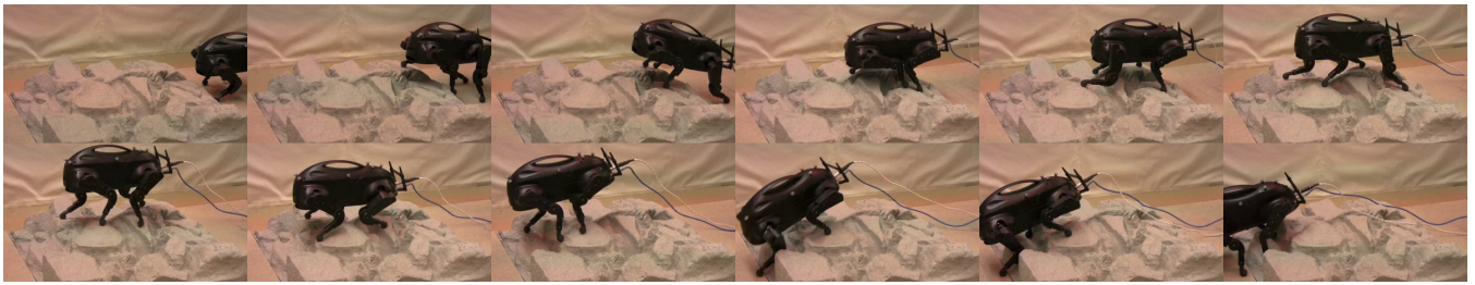
Fig. 4. Sequence of snapshots of the quadruped robot LittleDog crossing the test terrain after template learning. (left to right, top to bottom)
