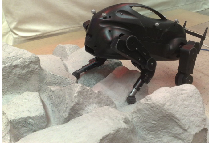
Fig. 1. The quadruped robot LittleDog and a sample terrain to be crossed.
