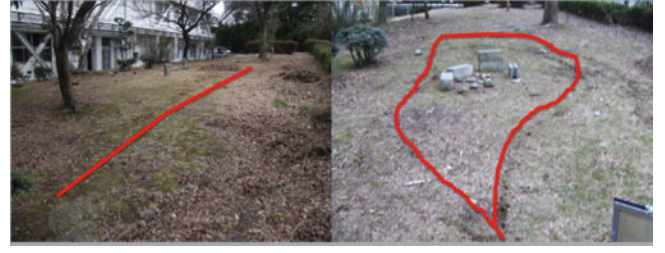
Fig. 3. Experimental fields: Field A is a slow ascent field (the left picture), Field B has an undulations and several blockades (the right picture). The red solid lines in the both pictures are the rover trajectories in the experiments.
