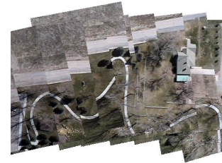
Fig. 1: This image sequence demonstrates the noisy pose estimations in MAV Video Sequences. Note how inaccuracies in the pose estimates cause discontinuities in the global mosaic.
