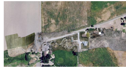
Fig. 5: Geo-referenced mosaic of Vineyard in Utah created using the optimized pose estimates. The geo-locations in this mosaic are 7m or less.
