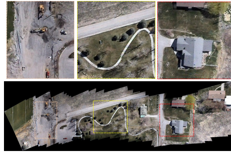
Fig. 4: This figure shows the quality of an actual MAV mosaic created using 600 MAV images of Vineyard in Utah.
