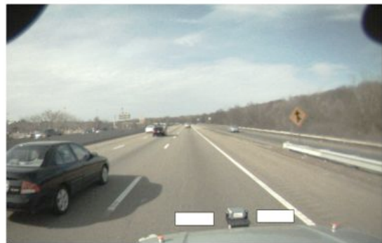
Fig. 1. A scene taken from the camera mounted on the car. The two white boxes represent the sampling regions close to the car where other objects should not lie. The pixels in these regions are randomly sampled.
