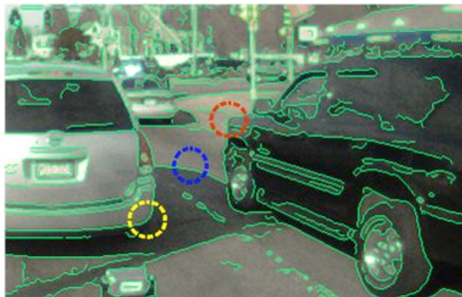
Fig. 3. The edge detection result of a frame. Three types of boundaries are shown (blue: shadow and road, red: road and dark, yellow: shadow and bright).
