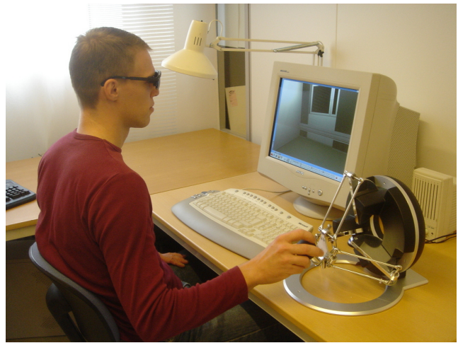
Fig. 6. User interface hardware configuration, with a CRT stereo display, an Omega haptic device, and a loudspeaker.
