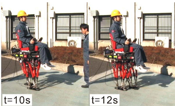
Fig. 12. Walking experiment outdoors with 7 degrees inclination. The walking cycle is 2.0 s/step with a step length of 200 mm/step.
