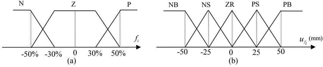
Fig. 4. (a) membership functions of  $f_i$  ( $i=1,2,3,4$ ) in the force rule base, (b) membership functions of  $u_{f_i}$  ( $i=1,2,3,4$ )
