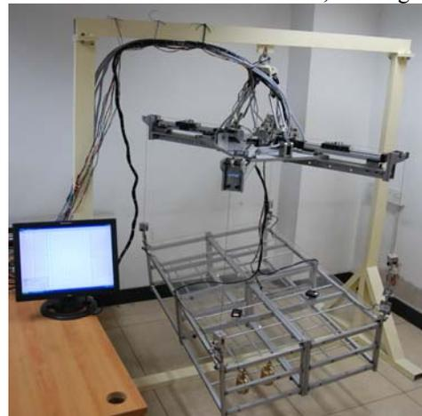
Fig. 1. The cable-driven auto-leveling parallel robot
