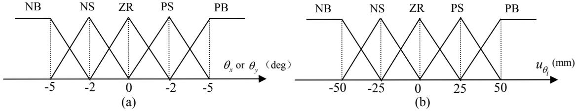
Fig. 5 (a) membership functions of  $\theta_x$  and  $\theta_y$  in the angle rule base, (b) membership functions of  $u_{\theta_i}$  ( $i=1,2,3,4$ )
