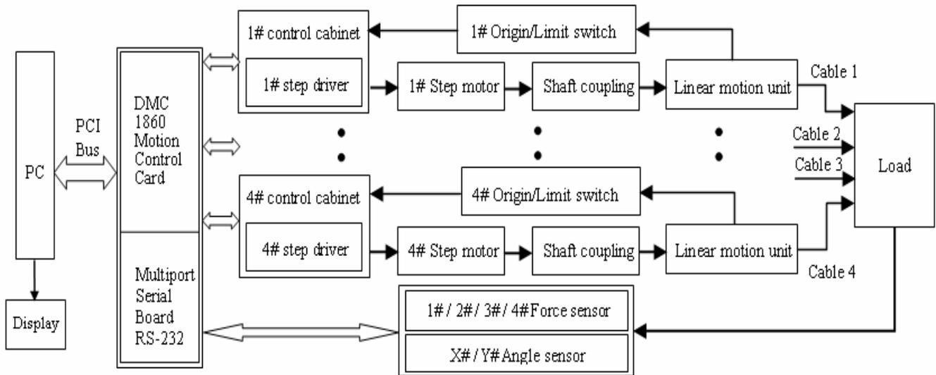
Fig. 2. Architecture of the closed-loop control system
