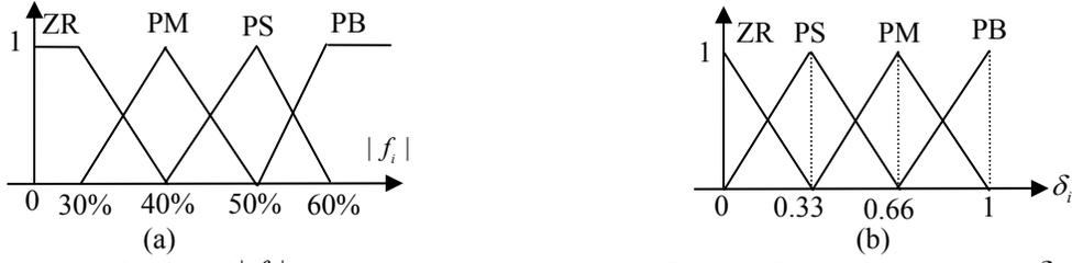
Fig. 6(a) membership functions of  $|f_i|$  in the high level layer, (b) membership functions of the coordination operation  $\delta_i$  ( $i=1,2,3,4$ )
