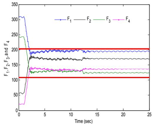
Fig. 7. Adjustment curves of leveling adjustment and force tuning.
