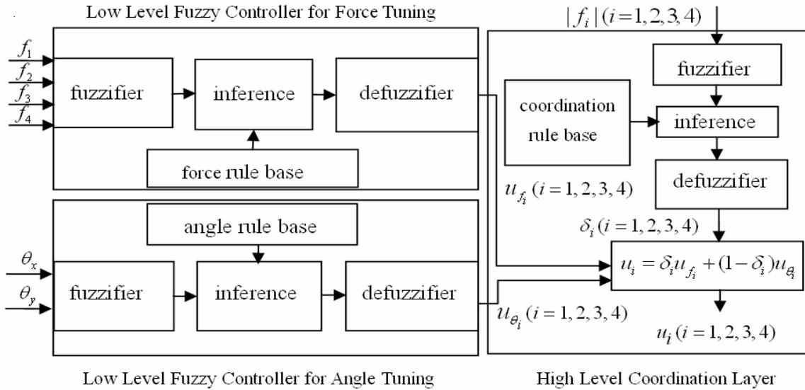
Fig.3. Structure of the hierarchical fuzzy controller
