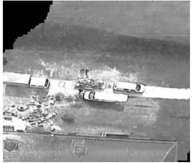
Fig. 1. An image map generated with iFMI in real-time from about 300 images acquired with an UAV. The scene involves several challenges, especially large featureless areas.
