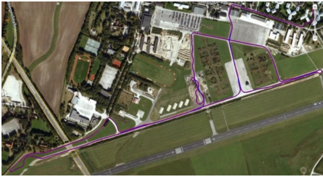
Fig. 10. Map view of the driven convoy scenario (blue: leader path, red: follower path). The total length of the track is 5937m, driven at an average speed of 6.9m/s, with 17.7m/s top speed. Both vehicles' position and heading were measured for reference by two Inertial Navigation Systems (INS) with D-GPS accuracy (aerial image: Google Earth).
