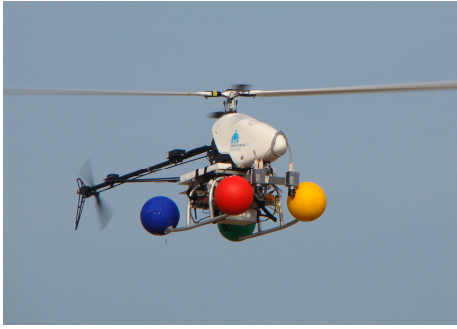
Fig. 1. Helicopter testbed Colibri III, during a flight. Color landmarks onboard the UAV are used as key features for the position estimation algorithm.
