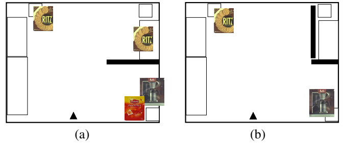
Fig. 13. Two experimental settings. Small rectangles indicate desks and shelves. Black bold lines indicate partition walls which may occlude objects. Objects to detect are put on desks.
