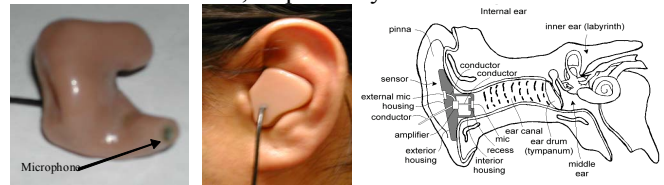
Figure 3: Earpiece containing the microphone, Earpiece placed in the ear of a subject, Graphic of earpiece inserted in the ear canal
