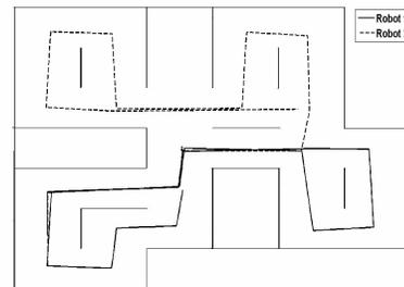
Fig. 6.. Trace of robots for complete sensor-based coverage
