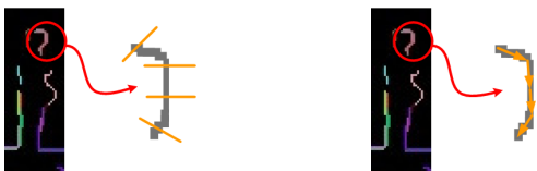
Fig. 4. The two types of edge descriptors used in our detection algorithm. Left: Histogram of orientations: for each edge point of a segment we use the orientations of the corresponding gradient, here shown in yellow on four sample edge points, and compute a histogram over them. Right: Vector of line segment orientations: From a polyline approximation to the edge segment, here shown as yellow arrows, we store the orientation angles of each line segment in a vector.
