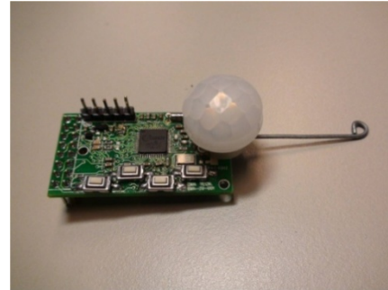
Fig. 4 The experimental platform integrated with CC2431 and pyroelectric sensor
