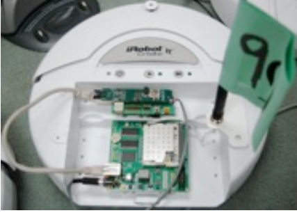
Fig.5. A radio node built by iRobot Create with Ubiquiti radio module and Gumstix Verdex.
