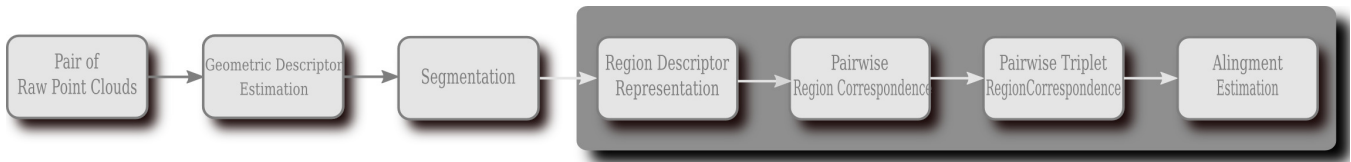
Fig. 1: Region-based global registration algorithm pipeline. This paper contributes the outlined stages of the global registration pipeline.
