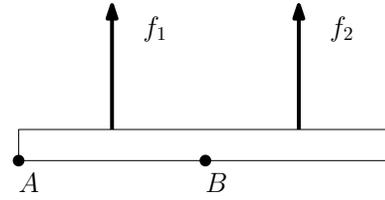
Fig. 2: Choices of origin resulting in different torque.
