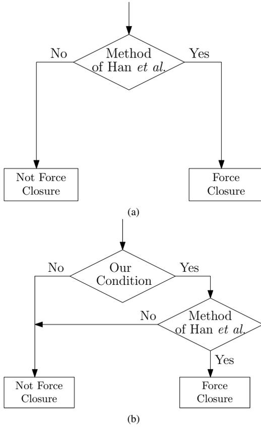
Fig. 4: Flowchart of force closure testing method. (a) The method of Han *et al.* (b) The method of Han *et al.* with our condition (described at the end of Section III) as a filtering criteria.
