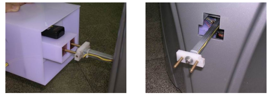
Fig. 3. (a) Docking station. (b) The robot docking mechanism which is under servo control.
