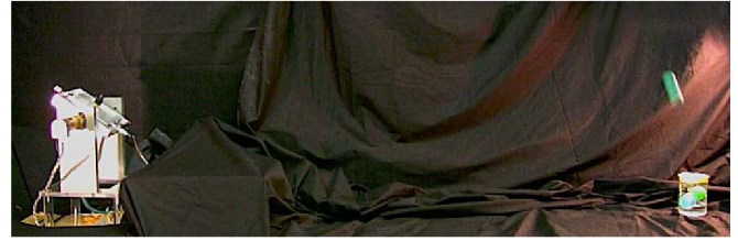
Fig. 11. Long-range ballistic positioning of spheres. Note the sphere falling towards the target beaker on the right.
