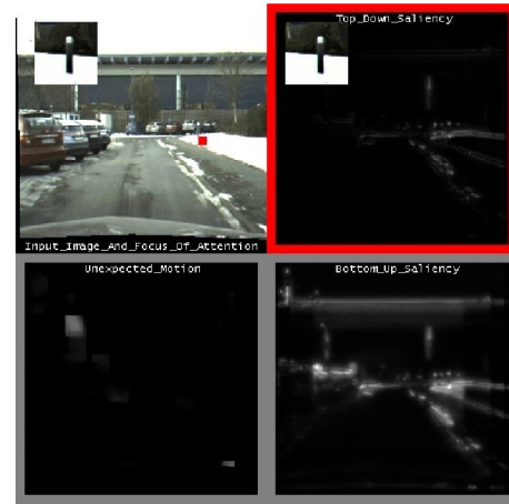
Fig. 5. Frame 2. Initially, the system focuses its attention on the poles along the road (upper left). This is task-driven and relies on the top-down saliency (upper right), as indicated by the red box. Bottom-up saliency (lower right) and ventral attention (lower left) are running in parallel, but do not yet influence the focus of attention.
