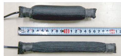
Fig. 5. McKibben pneumatic artificial muscle : contraction as air supplied (above) and expansion as air exhausted (below)
