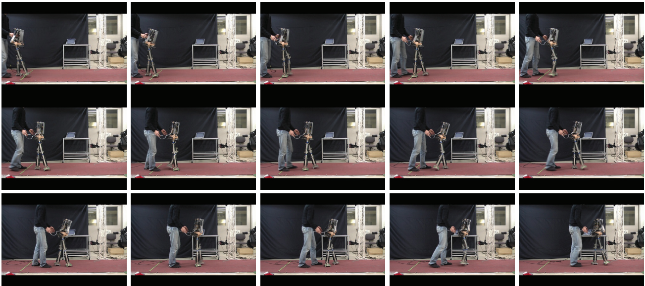
Fig. 12. Walking behavior of Pneumat-BT with extra load ( P_a = 0.40 MPa)
