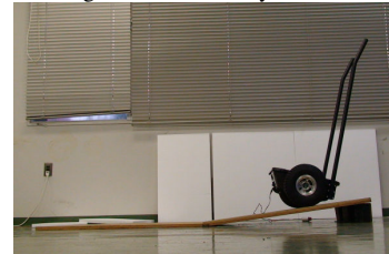
Fig. 4. state C: the vehicle maintains a balanced posture and stands still
