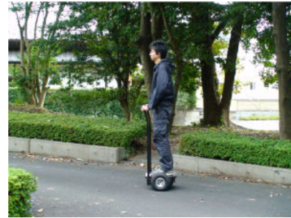
Fig. 1. Moving human-riding-type wheeled inverted pendulum vehicle on slope
