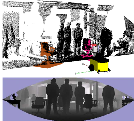
Fig. 1. Three-dimensional point cloud recorded with a mobile robot (top) and the corresponding range image (bottom). In the point cloud we also highlight two chairs identified with our approach.
