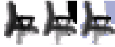
Fig. 4. Range image as it should look like according to the model (left) and actual part of the scene range image (middle). The black part on the top right of the image is clutter in front of the object. The right image shows the overlay of the other two images. The parts that are too different are marked in blue.
