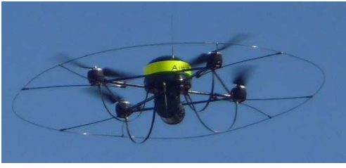
Fig. 1. AR-100 with camera mounted underneath the flight board.
