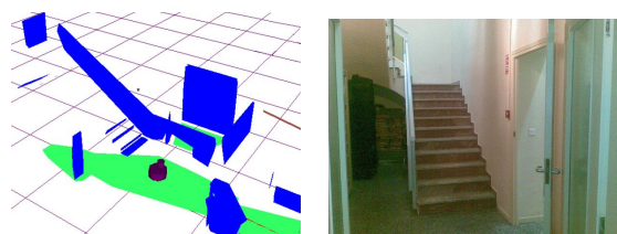
Fig. 5. Left: detailed scene of the 3D map of our laboratory. Right: the actual environment.
