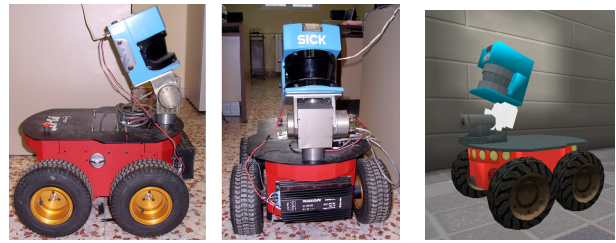
Fig. 1. Left:3D data acquisition system, mounted on our robot Nemo. Right: The USARSim Nemo's model we have built
